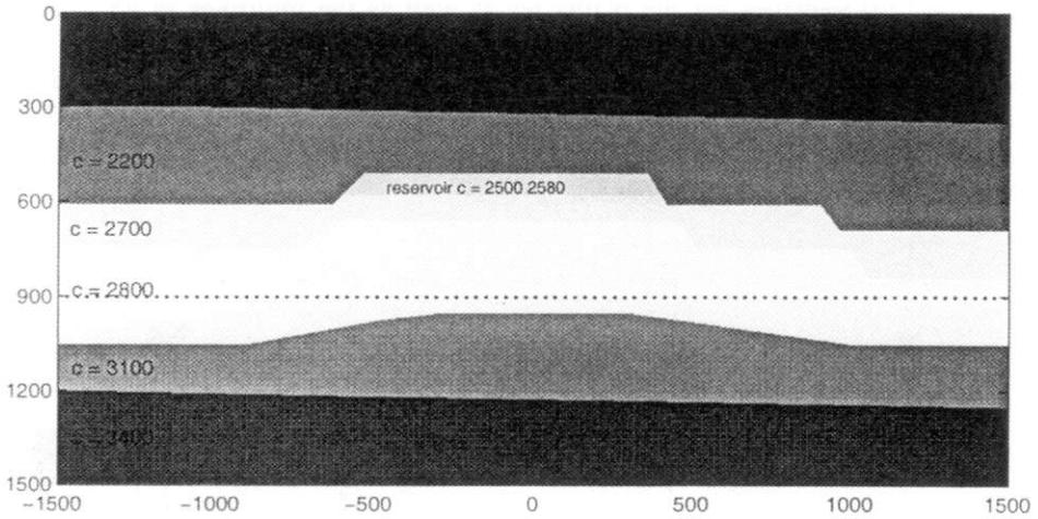
Fig. 7. Subsurface model, including a reservoir in which changes take place:  $c_A = 2500$  m/s,  $c_B = 2580$  m/s. The boundary integral (20) is evaluated at  $x_3^2 = 900$  m.
