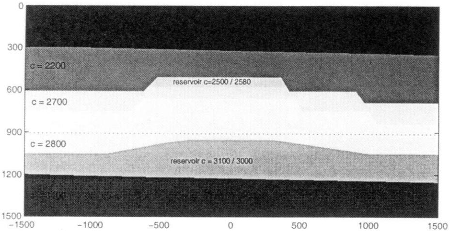
Fig. 10. Subsurface model, including two reservoirs in which changes take place. Reservoir 1:  $c_A = 2500$  m/s,  $c_B = 2580$  m/s. Reservoir 2:  $c_A = 3100$  m/s,  $c_B = 3000$  m/s. The boundary integral (20) is evaluated at  $x_3^2 = 900$  m.
