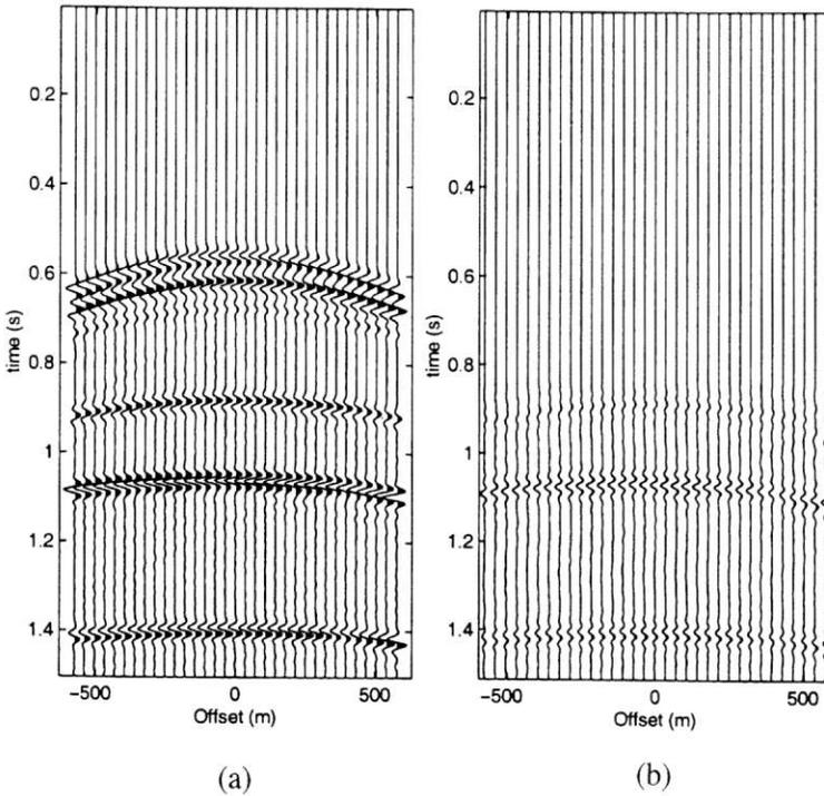
Fig. 11. Results for the stacked reservoir model of Fig. 10. (a) Difference of two shot gathers, contaminated by traveltime differences. (b) Evaluation of the boundary integral (20). This result contains the true time-lapse changes of the reflectivity of the second reservoir.
