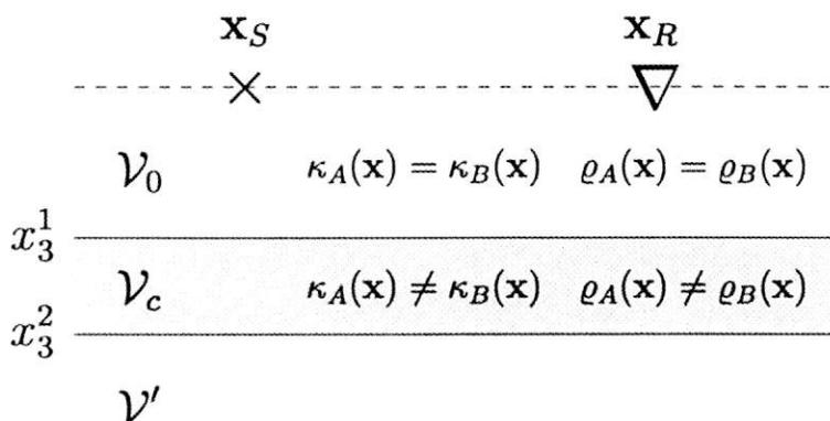
Fig. 4. Configuration for the time-lapse seismic method.
