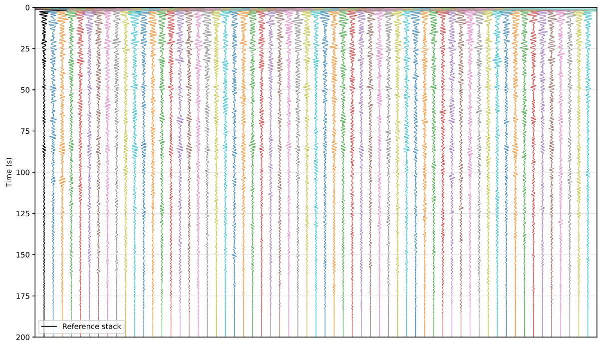
Fig. B.1. Reference linear stack computed using all available autocorrelations (black), compared with subsampled linear stacks obtained from random subsets of autocorrelations (colored).
