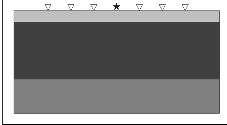
Figure 3.8: Configuration of a horizontally layered medium.
