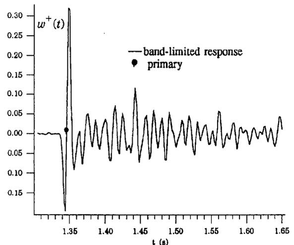
Fig. 1 Exact band-limited transmission response of a well-log with a large primary transmission loss, convolved with a Ricker wavelet (250Hz).
