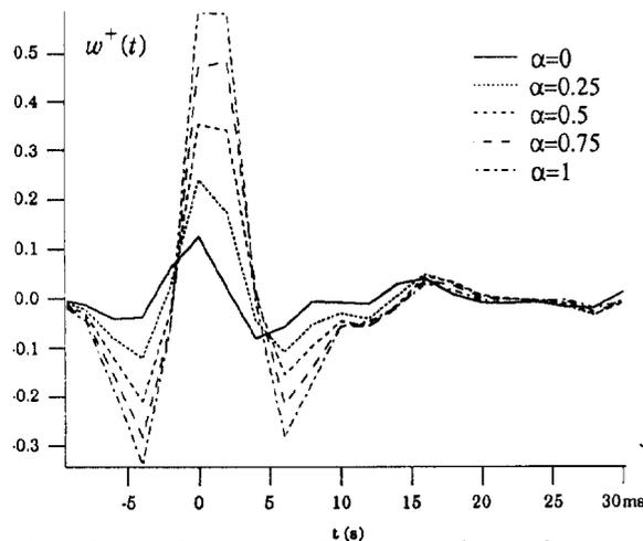
Fig. 5 Band-limited transmission responses for a medium defined by FGN with  $0 < \alpha < 1$
