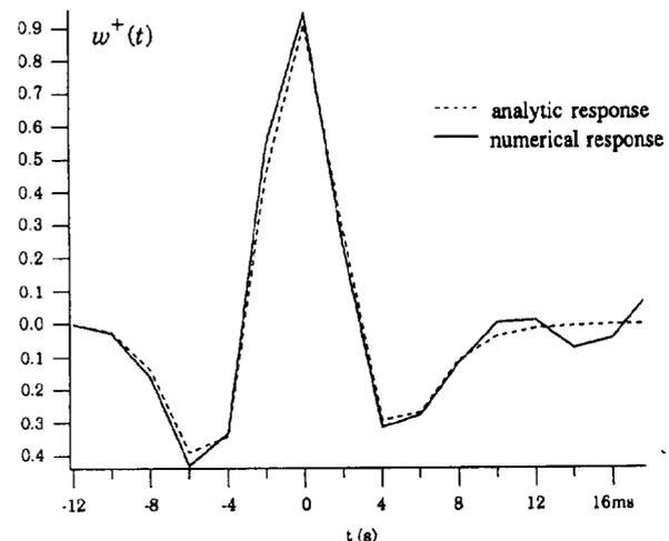
Fig. 6 Comparison of the exact transmission response and its analytic approximation eq. (5)
