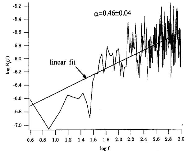
Fig. 4 Estimate of the log-log power spectrum of the reflection coefficients yielded by the log of Fig. 3,  $\alpha=0.46\pm 0.04$
