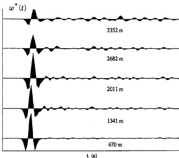
Fig. 2 Band-limited transmission responses; the primary travel times have been corrected for the various depth levels
