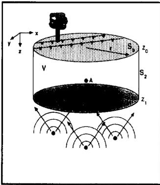
FIG. 1. Geometry for Kirchhoff integral in seismic situation; pressure in  $A$  is computed from measurements on surface of volume  $V$ .
