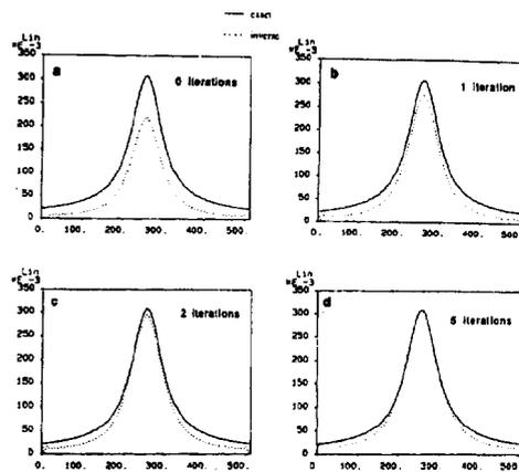
FIG. 5. Amplitude cross-sections as a function of trace number for inverse extrapolated result (dotted line) and the exact result (solid line). (a) With 0 iterations, amplitude shows a considerable discrepancy (30%); (b) with 1 iteration, discrepancy has largely been reduced; (c) with 2 iterations, amplitude has improved again; and (d) with 5 iterations, there is almost a perfect match. Discrepancy at large offsets is due to negligence of evanescent waves.
