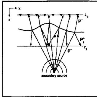
FIG. 2. Since scattered wave-field  $P_s^+$  cannot be measured in practice, it is always neglected, thereby introducing second-order amplitude errors.
