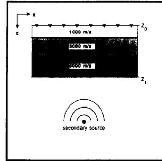
FIG. 3. Example shows principle of iterative approach; acoustic subsurface model containing two reflectors with strong velocity contrasts (density constant).
