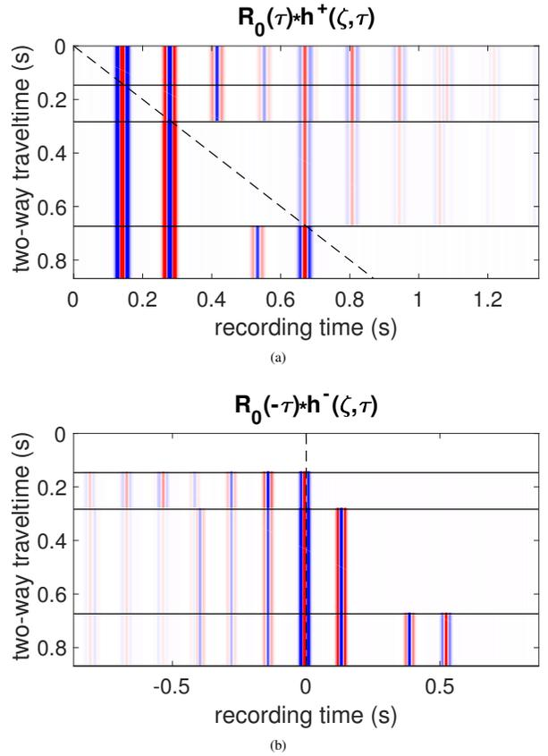
Figure 1: Reflection response (a) convolved with  $h^+(z_0, \zeta, \tau)$  and (b) correlated with  $h^-(z_0, \zeta, \tau)$ , as a function of two-way traveltime  $\zeta$  and recording time  $\tau$ .
