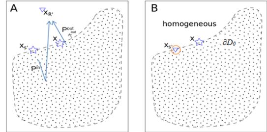
Figure 2. Configurations of state A and B for inter-source SI by MDD. The dotted line describes the boundary  $\partial D$  enclosing the volume,  $D$  and  $\partial D_0$  is the virtual receiver surface. The orange circle denotes the virtual receiver. The star denotes source and the triangle denotes receiver.
