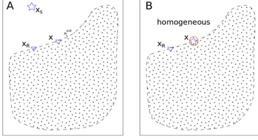
Figure 1. The configuration of state A and B for inter-receiver SI by MDD. The dotted line describes the surface boundary  $\partial D$  enclosing volume  $D$  and  $\partial D_0$  is the virtual receiver surface. The orange circle denotes the virtual source. The star denotes source and the triangle denotes receiver.
