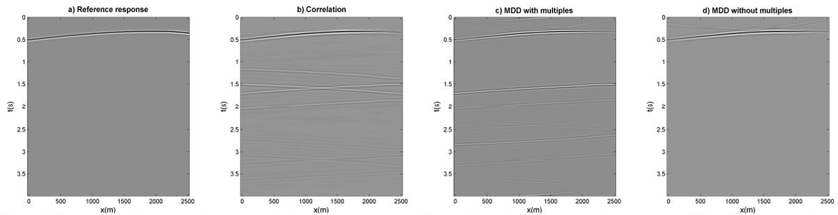
Figure 4. Shot gathers of the retrieved responses and the reference response. a) The modeled reference response of a source at  $x=1370$  m. The direct arrivals are removed. b) The response obtained by CC. c) The response obtained by MDD when the multiples are not separated in the input. d) The response obtained by MDD when only the direct wave and the primary reflected wave are used as input.
