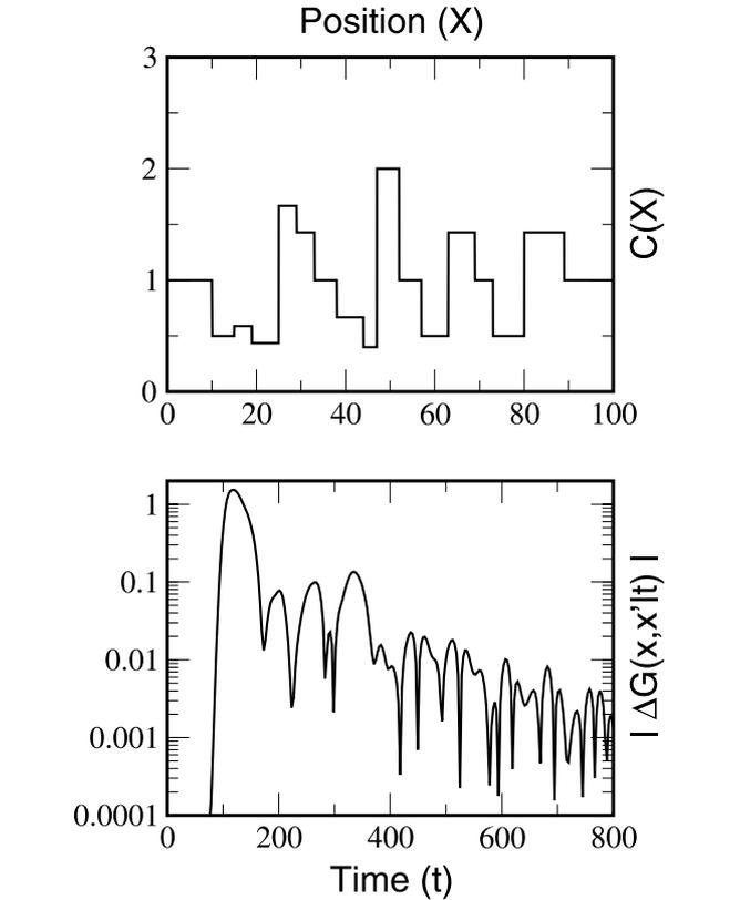
Fig. 3. Time-domain response function of a randomly layered system. The top graph shows the position-dependent velocity  $c(x)$  and the lower one the corresponding response functions in a linear-log scale. The variables  $x$  and  $x'$  represent the detector and source position, respectively.
