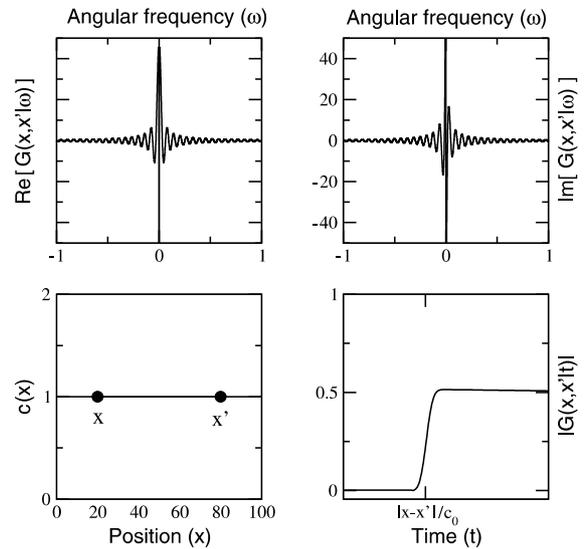
Fig. 1. Calculated response function for free propagation in 1-dimension. The top graphs show the frequency domain for the real (left) and imaginary (right) parts of the Green functions. The lower left graph shows the velocity profile and the lower right is the time-domain response function. Notice the agreement with the analytical results (see text). The variables  $x$  and  $x'$  represent the detector and source position, respectively.
