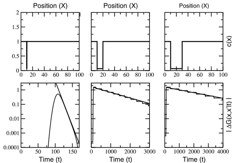
Fig. 2. Time-domain response function of a homogeneous ( $c_0$ ) system separated by a finite insertion ( $c_1 \neq c_0$ ) of different sizes. The top graphs show the position-dependent velocity  $c(x)$  and the lower ones the corresponding response functions in a linear-log scale. The straight lines are analytical expressions based on the lowest-order pole approximation (see text). The variables  $x$  and  $x'$  represent the detector and source position, respectively.
