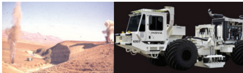
Fig. 1: Traditional seismic acquisition on land is done with dynamite or seismic vibrators
