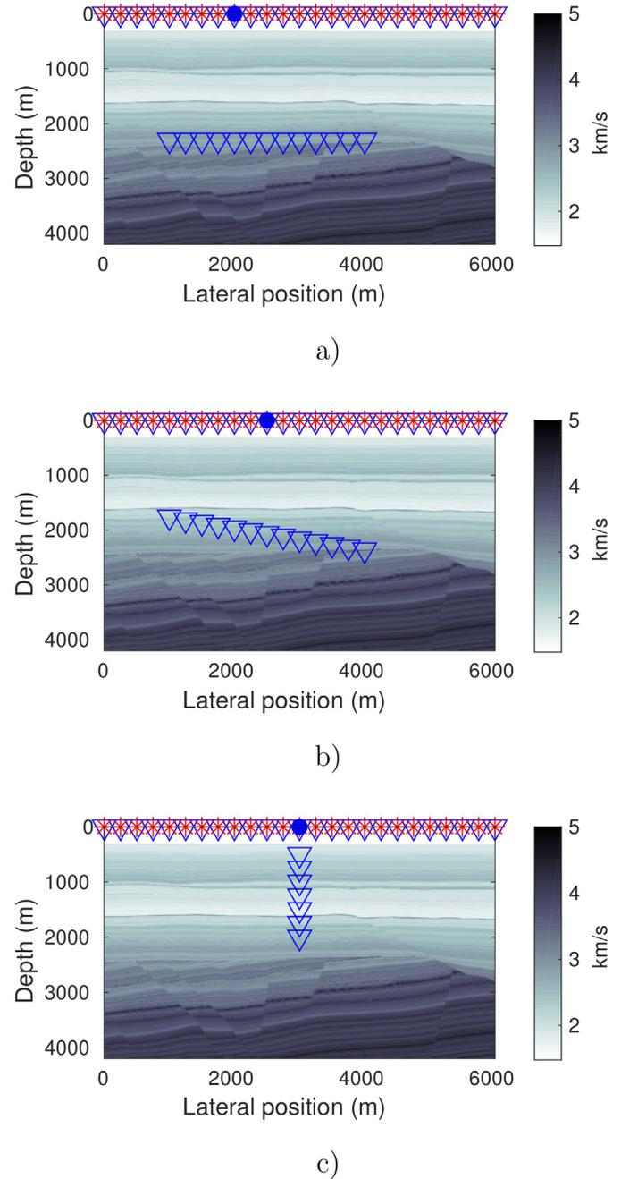
**Fig. 4.** The P-wave velocity model and the acquisition geometries for the a) horizontal borehole, b) deviated borehole and c) vertical borehole. The stars denote the sources in both the surface and borehole data, and the triangles denote the receivers. The blue circles denote the reference source positions, where the retrieved one-way wavefields are shown. (For interpretation of the references to colour in this figure legend, the reader is referred to the web version of this article.)
