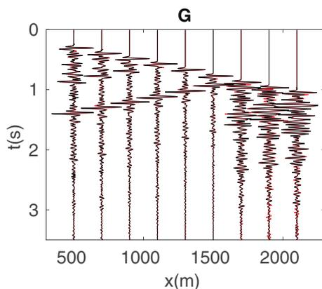
**Fig. 15.** Vertical borehole case. The comparison of the retrieved total wavefield ( $U + D$ , in black) and the recorded pressure field (in red) in borehole. (For interpretation of the references to colour in this figure legend, the reader is referred to the web version of this article.)
