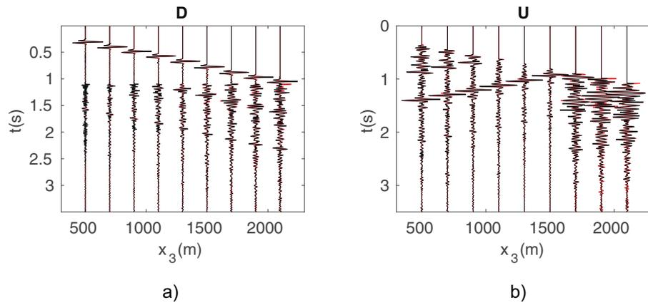
**Fig. 16.** Vertical borehole case. The comparison of the retrieved wavefields (in black) of a source at  $x_1 = 3000$  m at the surface. They are compared to those by standard PZ summation (in red). a) The downgoing field. An amplitude gain of a factor of 8 is applied on the events after the direct arrivals. b) The upgoing field. Every sixth trace is plotted. (For interpretation of the references to colour in this figure legend, the reader is referred to the web version of this article.)
