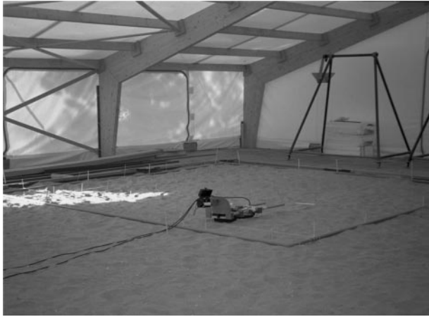
FIG. 4. The 3 \times 4 m test area within which the multicomponent measurements were made.
