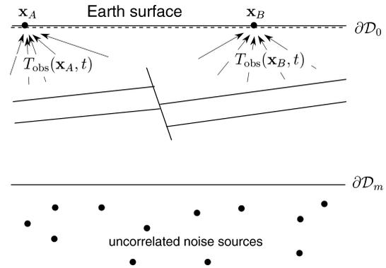
FIG. 3. Transmission response, observed at  $\mathbf{x}_A$  and  $\mathbf{x}_B$ , resulting from a distribution of uncorrelated white noise sources. According to equation (16), their crosscorrelation yields the reflection response observed at  $\mathbf{x}_A$  as if there were an impulsive point source at  $\mathbf{x}_B$ .
