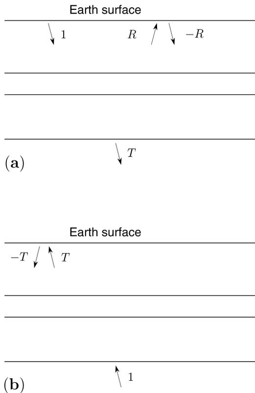
FIG. 1. (a) Plane-wave reflection response of a horizontally layered medium. (b) Plane-wave transmission response of the same horizontally layered medium.
